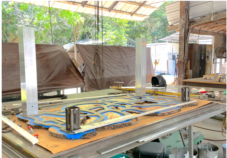
Figure 10: Assembly of legs onto the steel frame at Artsworld's shop
