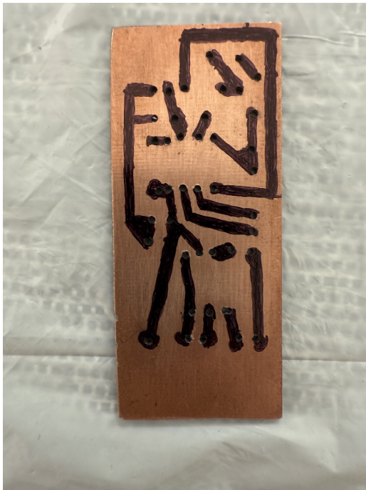
Figure 4: Masked Plate with Sharpie
